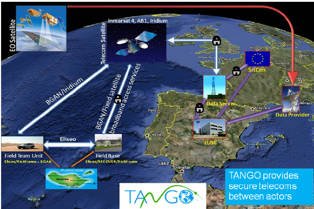
Satcom architecture of the evacuation demonstration of Madeira Island
